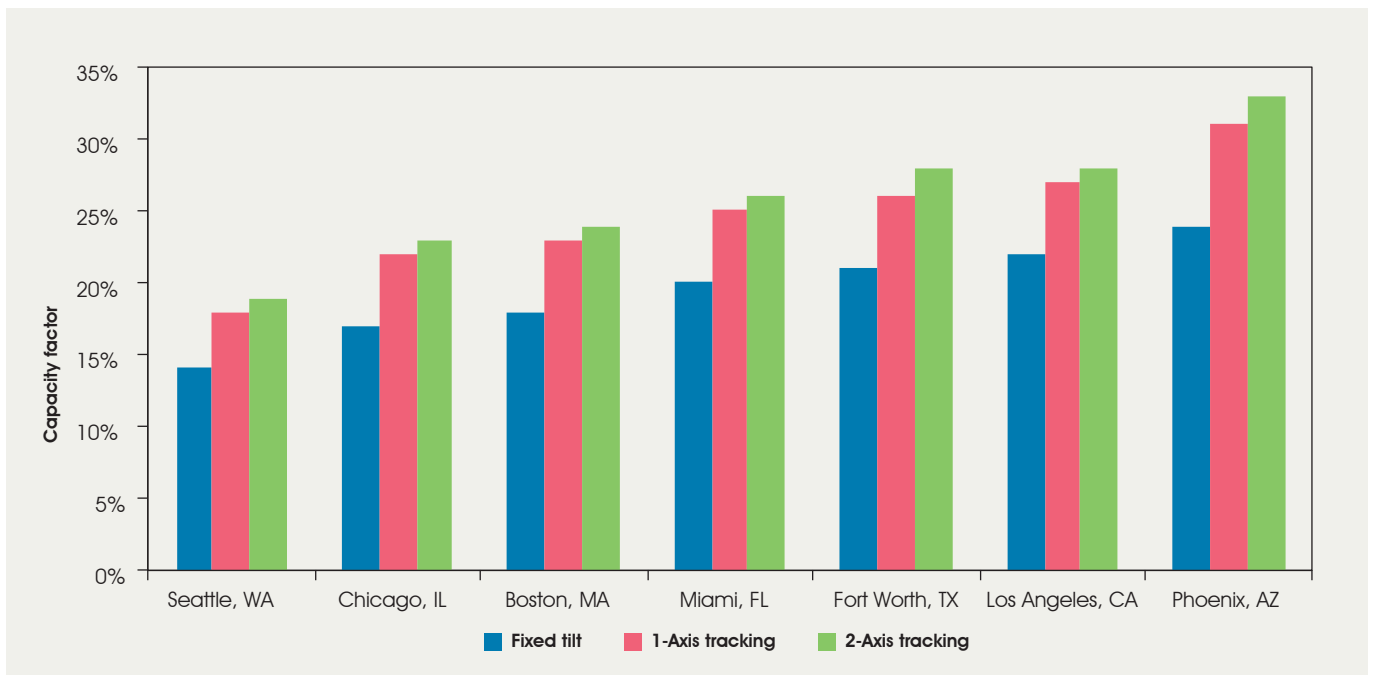
FIGURE 6.8: SOLAR PV SYSTEM CAPACITY FACTORS BY LOCATION AND TRACKING SYSTEMS IN THE UNITED STATES
