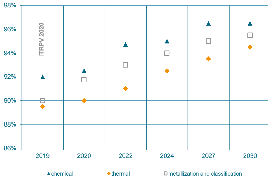
Fig. 70: OEE trend of state of the art new cell tools in new production facilities.
